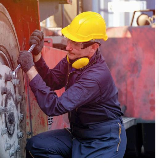
beefy as these specialised steel bolts are, they act like an elastic band, explains Gary Broadfield, director of Wheely-Safe. "If that band weakens or doesn't retain its elasticity, you won't get the frictional holding force on the back of the wheel nut." A tensile fracture - a break - is caused either by poor metallurgy of the stud in the first place, or over-torqueing, or repeated torqueing beyond the elastic point, he states.
